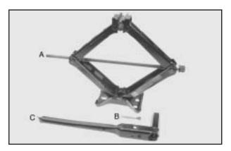
The tools you'll be using include the jack (A) extension and protector/guide (B) and wheel wrench (C).
